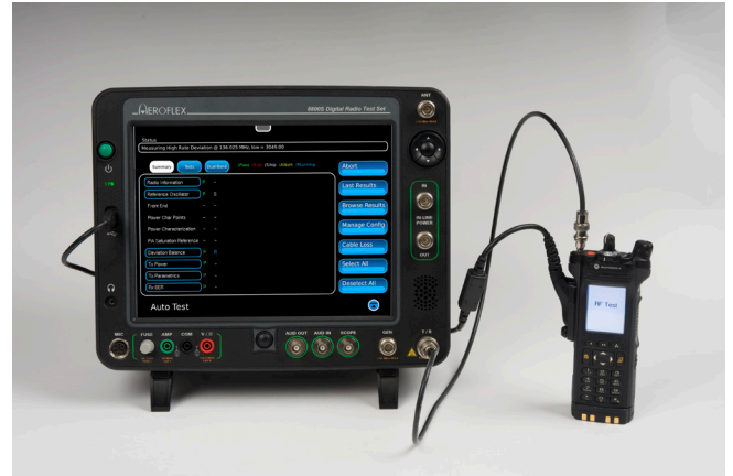
The 8800SX Auto-Test Setup
